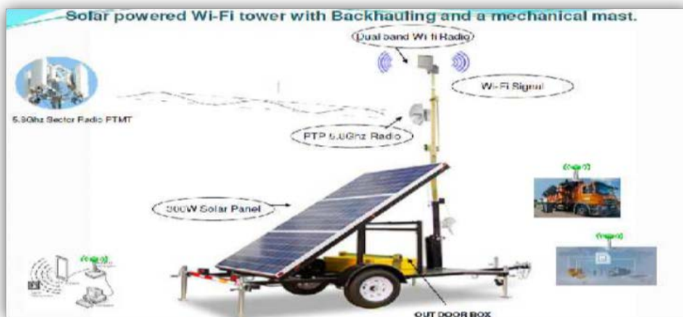
Fig. 7.5: Working mechanism of Solar Wi-Fi Trolley
