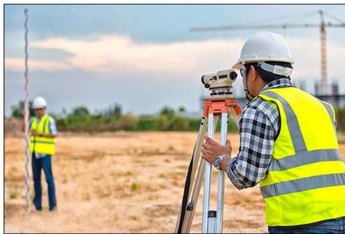
Fig. 5.4: Auto Level and Levelling Staff in the field
