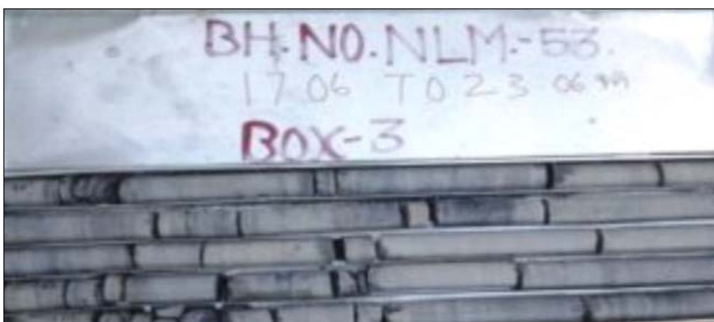
Fig. 1.21: Cores kept inside the boxes with proper marking
