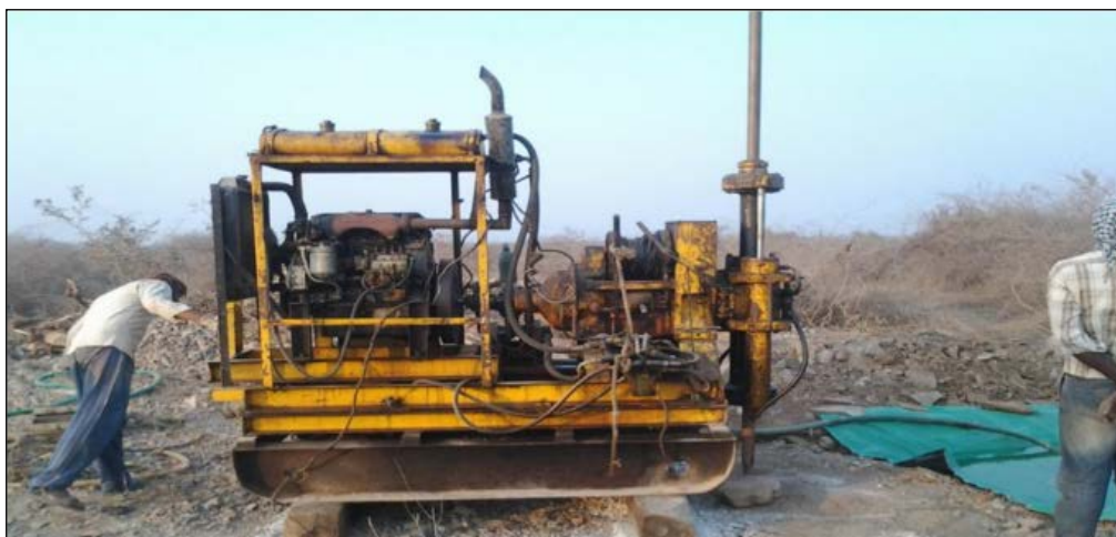
Fig. 1.19: Conventional Core drilling Method
