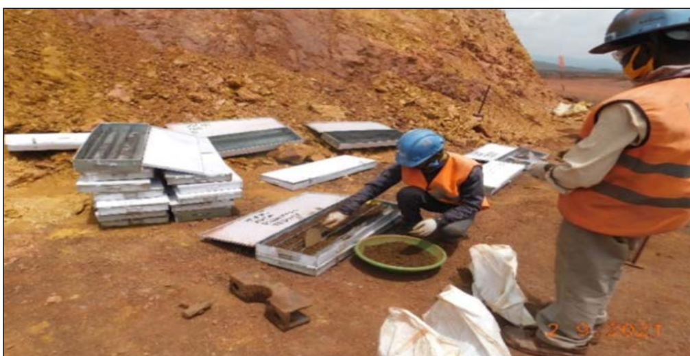
Fig. 1.20: Core boxes for keeping cores
