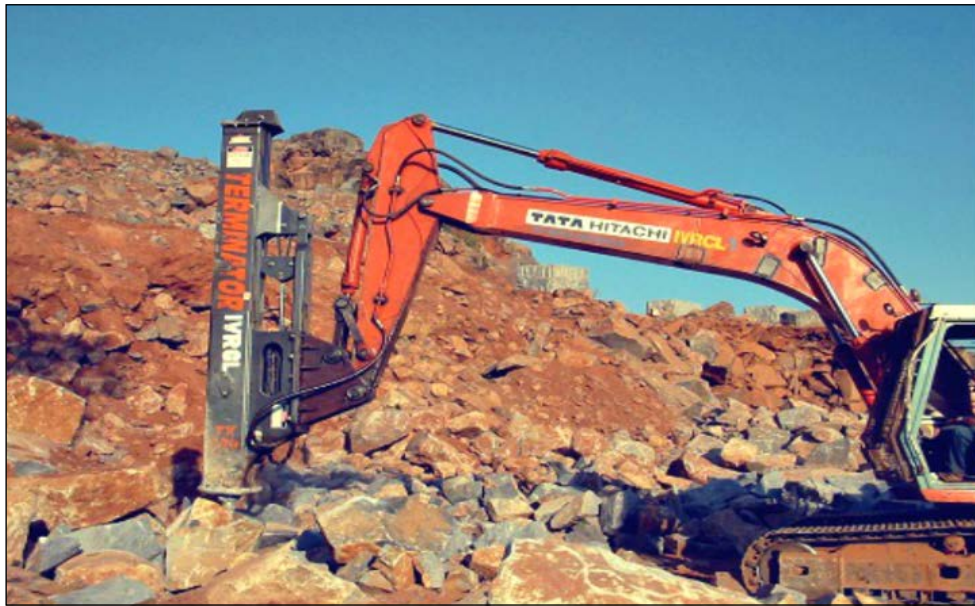
Fig. 2.23: Tata Hitachi Terminator Rock breaker
