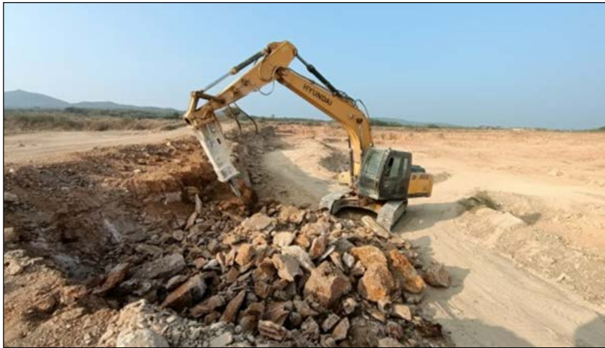
Fig. 3.10: Insitu Rock breaking Courtesy: Ishwaria Limestone Mines of M/s Tata Chemicals Ltd
