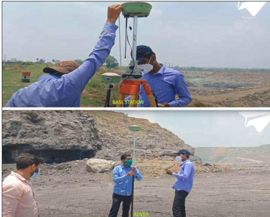
Fig. 5.14: DGPS survey in Open cast mine
