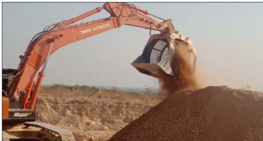
Fig. 3.13: 50mm Mesh Size Rotating Screen drum mounted on Excavator Courtesy: Ishwaria Limestone Mines of M/s Tata Chemicals Ltd
