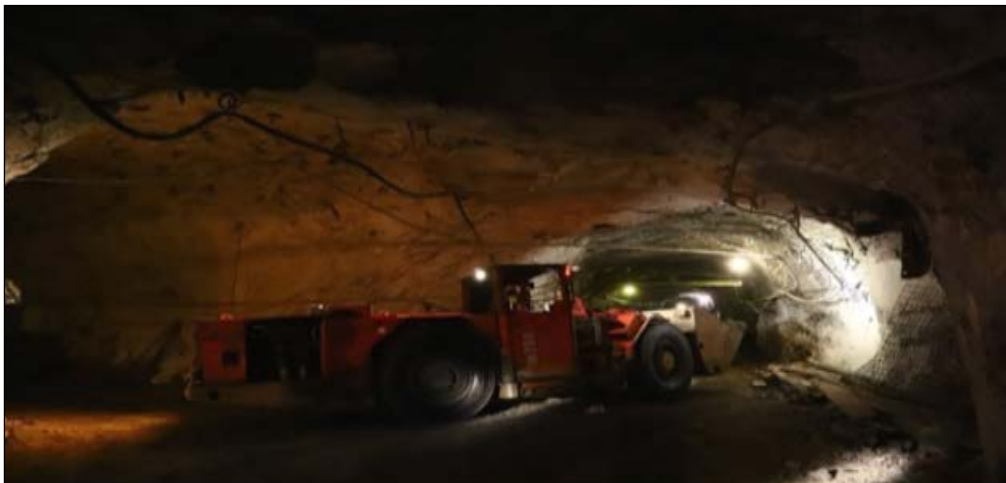
Fig. 3.9: Electrical-LHD- Operation of Load Haul Dump (LHD's) (electrical and diesel) in underground mines at Hutti Gold Mines
