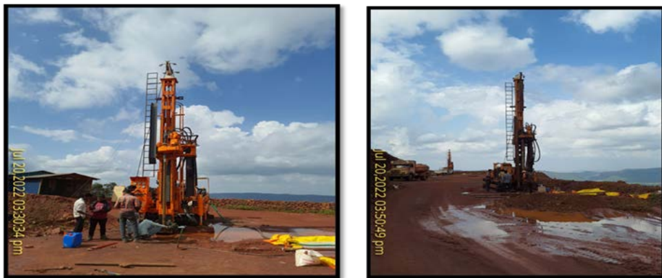
Fig. 1.23: Chain Mounted Diamond Core Drilling Machine Courtesy: Ramanadurga Iron Ore Mine of M/s. Sri K.S. Mineral Exports Pvt. Ltd
