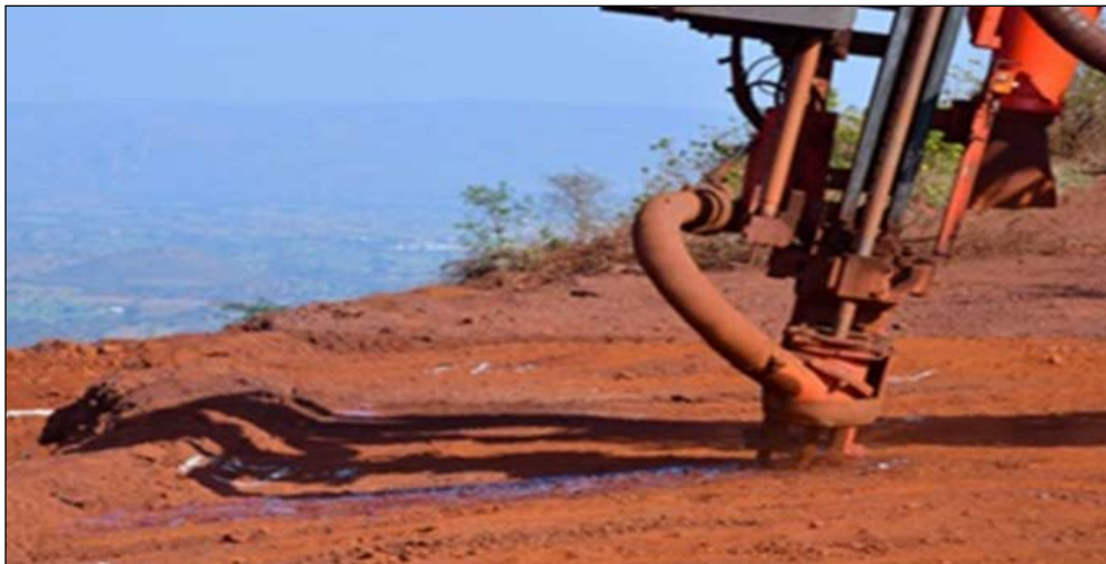
Fig. 1.5: Use of wet drilling technique
