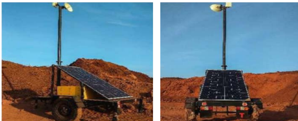
Fig. 7.6: Existing solar Wi-Fi trolley under operation at mine head
