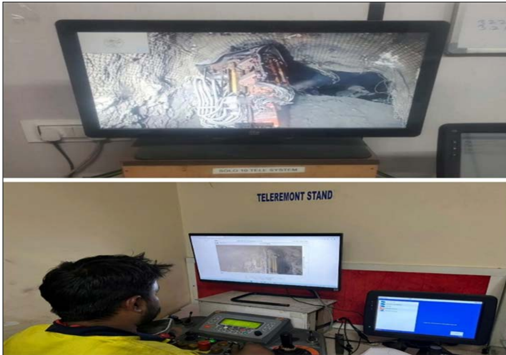
Fig. 1.9: Operator monitoring drilling operation from office
