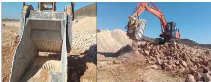
Fig. 3.11: Mobile Jaw Crusher mounted on Excavator Courtesy: Ishwaria Limestone Mines of M/s Tata Chemicals Ltd
