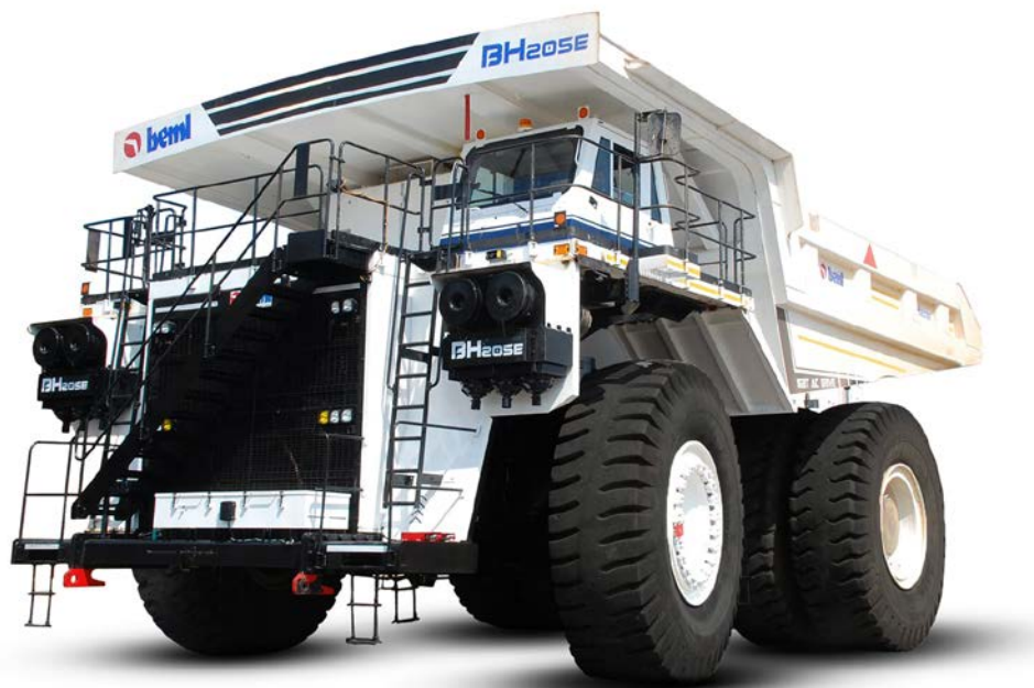
Fig. 4.1: Rear Discharge Dumper BH205E; India's Largest Indigenous Electric Drive Dumper
