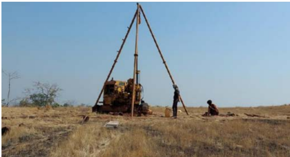
Fig. 1.18: Conventional Core drilling Method (Courtesy: Gudeghar Bauxite Mine)
