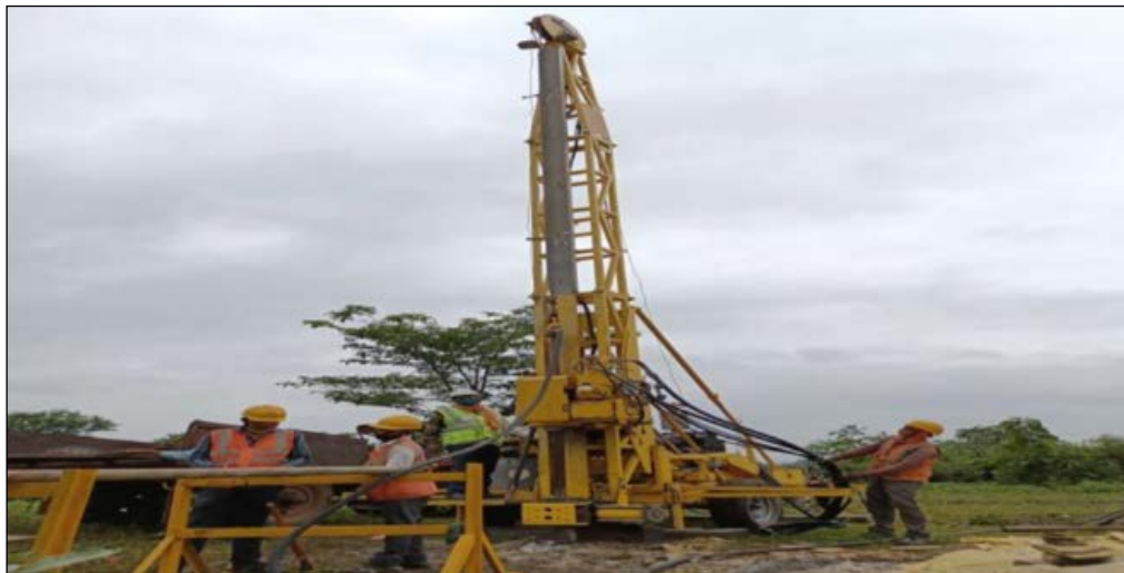
Fig. 1.24: Core Drilling Machine Model No. CS 1000 P4 (Atlas Copco, Series HQ, NQ (63.5 mm. & 47.67 mm)
