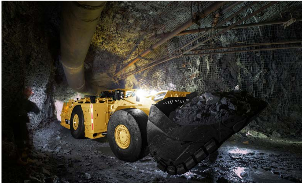
Fig. 3.6: Load Haul Dump: CAT Model R1700G
