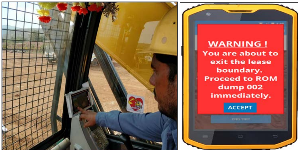
Fig. 1.15: Vehicle going out of the lease boundary - Real Time Alerts to Operators and Management
