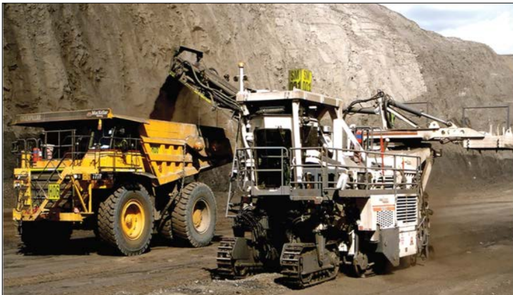
Fig. 3.16: Surface Miner operation
